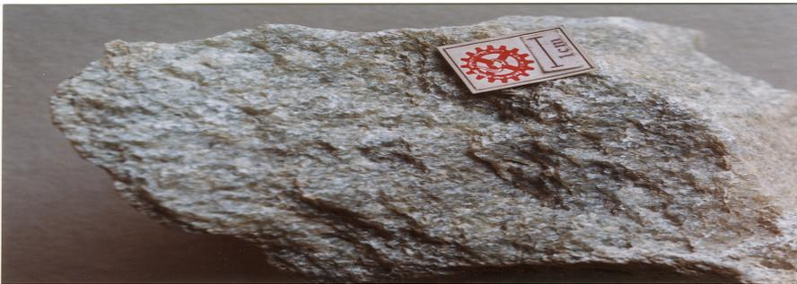
Fig. 1. Irregular and anhedral coarse grains of quartz and subhedral grains of altered feldspars are embedded in a matrix of pyrophyllite.
