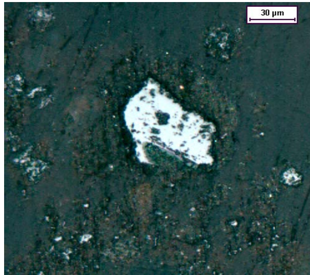
Fig. 5: Magnetite (white at the centre) is also observed in the head sample. It can be observed that there are numerous tiny inclusions of silicate gangue minerals within magnetite. Reflected light Microscopic photomicrograph.
