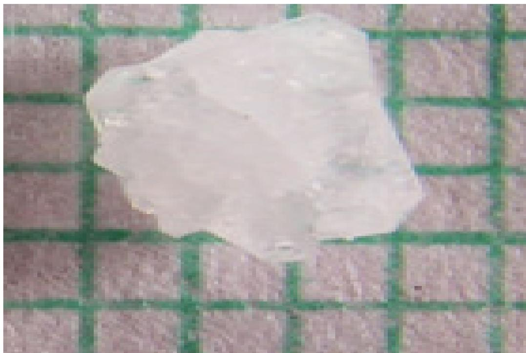
Fig.2. Harvested AMHP crystal in SDP.
