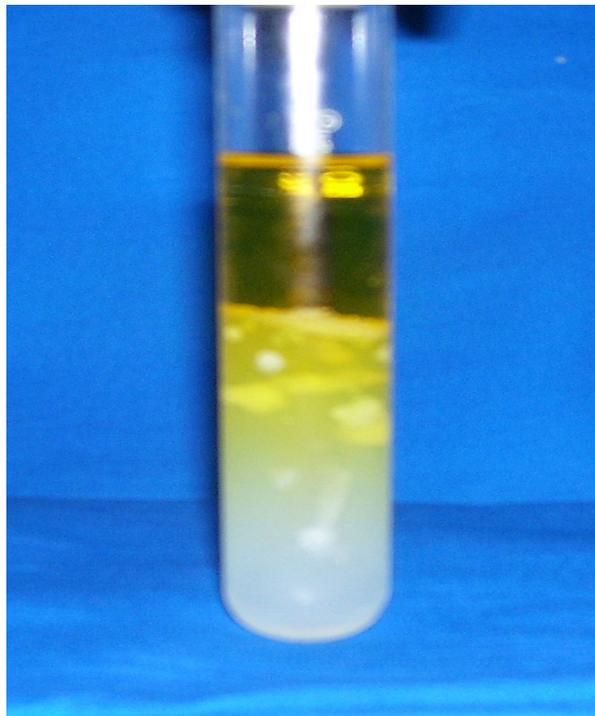
Fig -2. Growth of SrCrMHP crystal within laboratory environment (SDP).
