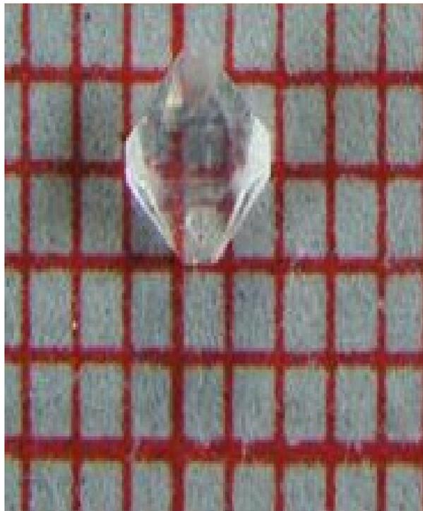
Fig-6. Harvested SrCrMHP crystals in DDP (3 mm x 3.5 mm x 3 mm).
