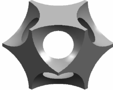
Figure 3: Spherical unit cell used to model the porous medium (Druma [2005])
