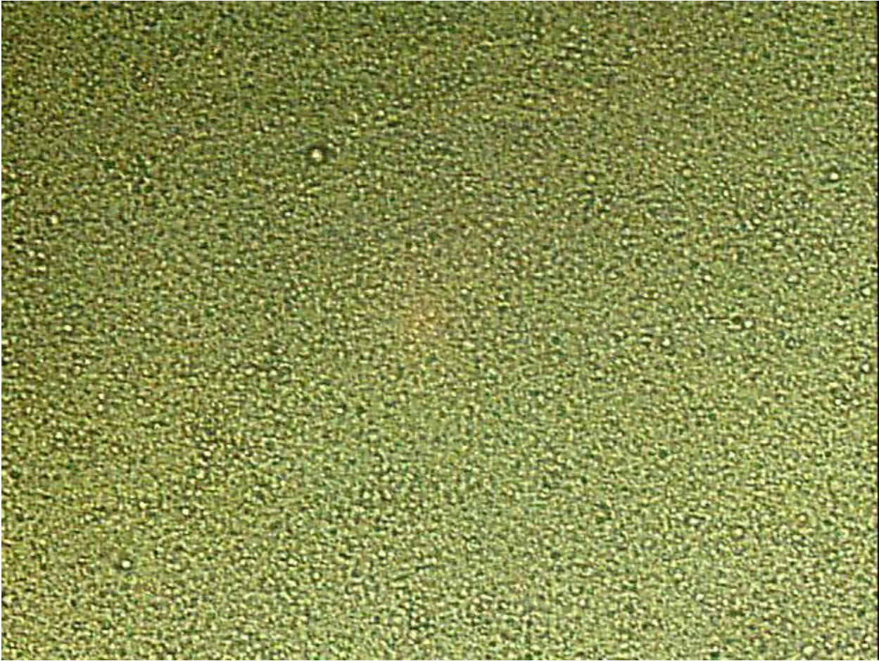
Figure 3. Optical micrograph of a surface of a VA/AA-based emulsion (6.6 wt % solids) at 400X magnification, showing a bicontinuous network structure with 5-10 \mu\text{m} open cells.
