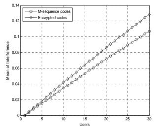
Figure 3. Comparing mean of interference M-sequence and encrypted codes in channel with 256 hop.
