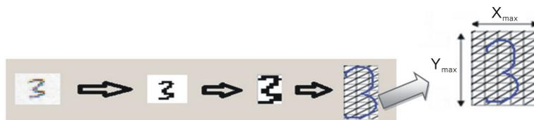
Figure 2. Example for input preparation for digit “3” and its coordinates.
