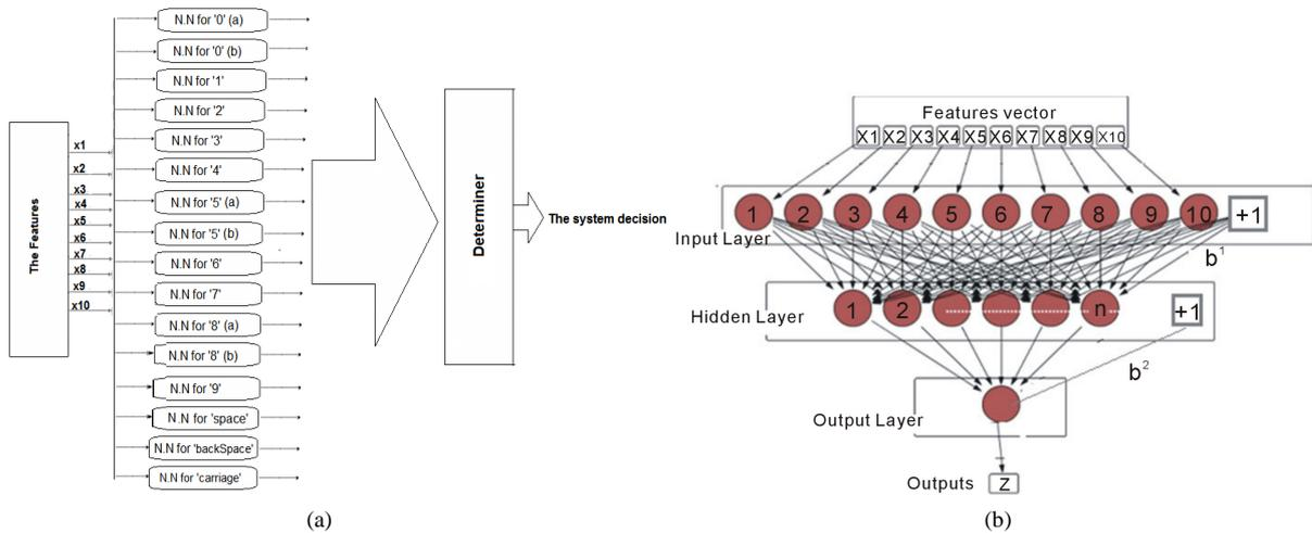
Figure 5. (a) Block diagram of PNN classifier; (b) one of neural networks of PNN classifier.
