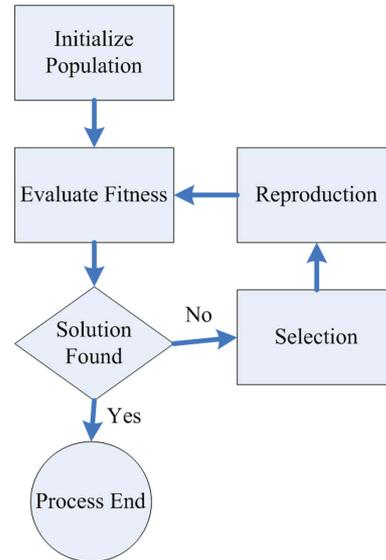
**Figure 4. Flow chart of genetic algorithm iteration.**
