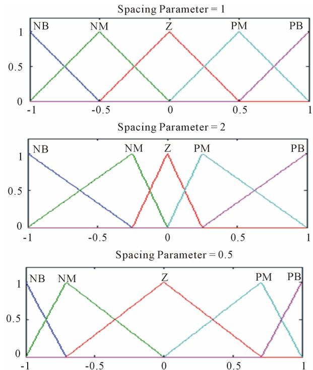
**Figure 2. Effect of spacing parameter on MFs.**
