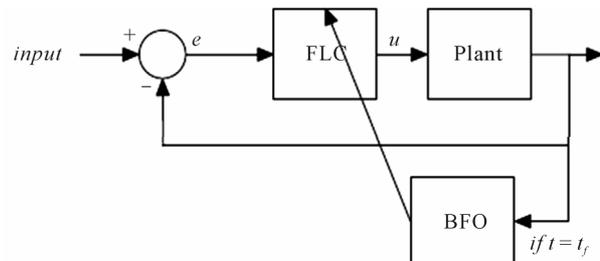
**Figure 4. Tuning of FLC parameters by BFO algorithm.**
