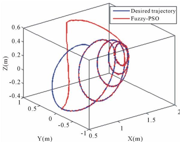
**Figure 9. Performance of FLC using PSO algorithm.**
