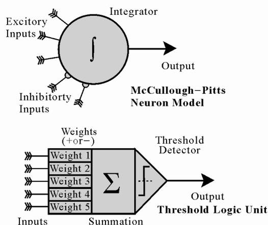
**Figure 3.** McCulloch and Pitts simplified model of a neuron and its implementation as a threshold logic unit [7].
