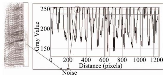
Figure 9. Description of noise and effect of applying cutoff level for *Hikari 52*.
