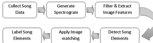
**Figure 4.** Process flow diagram of the songnote detection and recognition.
