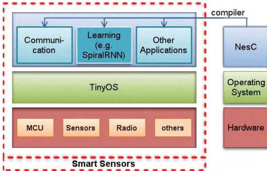
Figure 31. Structure of a typical smart sensor mote. TinyOS is the specific operating system for embedded system such as smart sensor and provides interfaces among hardwares and softwares. NesC language, as a compiler, compiles and builds softwares for different applications
