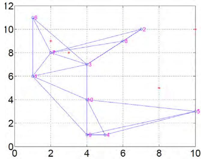
Figure 20. Simulation environment with sensors (numbered circles) and heat sources (stars). Also shown are the communication links between sensor nodes
