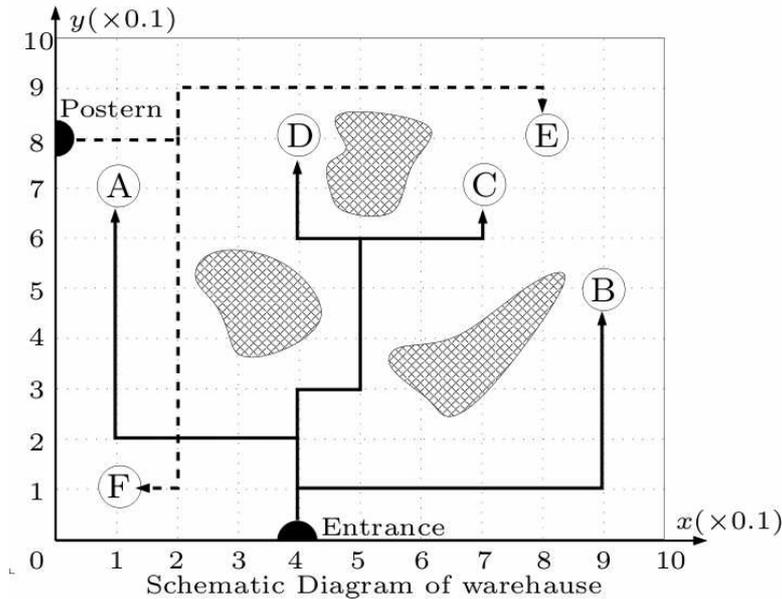
Figure 24. Application example “warehouse”: Depending on their type, newly delivered goods have to be stored in different areas labeled by A-F. The trajectories used by trucks are shown as well
