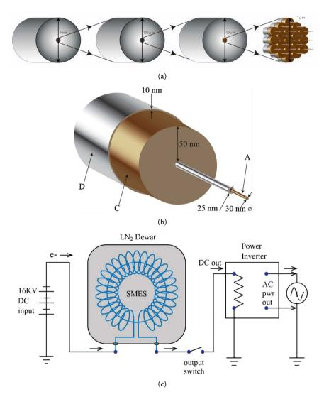
**Figure 2.** (a) Representation of multiple filaments in a cable where each 1 micron yields 19 nano filaments; (b) Detailed illustration of a nano wire filament; (c) SMES in an Energy Storage Application.
