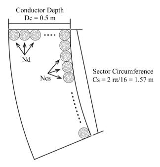
**Figure 7.** Conductor packing in each sector.
