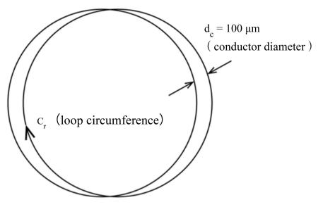
**Figure A-3.** Application area of Lorentz force for a single conductor loop in an SMES torus.
