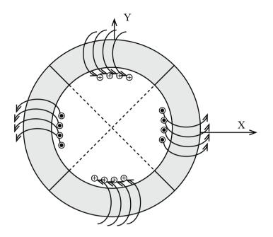
Figure 10. Quadrupole generation via torus alternating current (AC).
