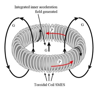
**Figure 1.** Gravitational force generation coil from Forward 1962 [1] with an inspiralling mass current, with a vector potential P, creating gravitomagnetic field G, which is additive in the center.
