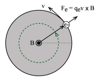
Figure A-1. Lorentz Forces due to Electron orbit in one loop of SMES.
