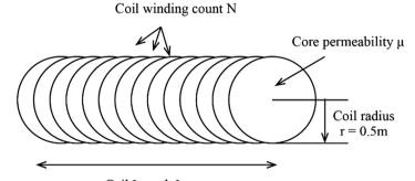
Coil Length I Figure 8. Geometry determining inductance.
