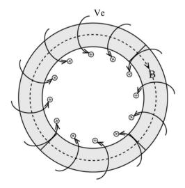
Figure A-2. Magnetic field in an SMES torus core.
