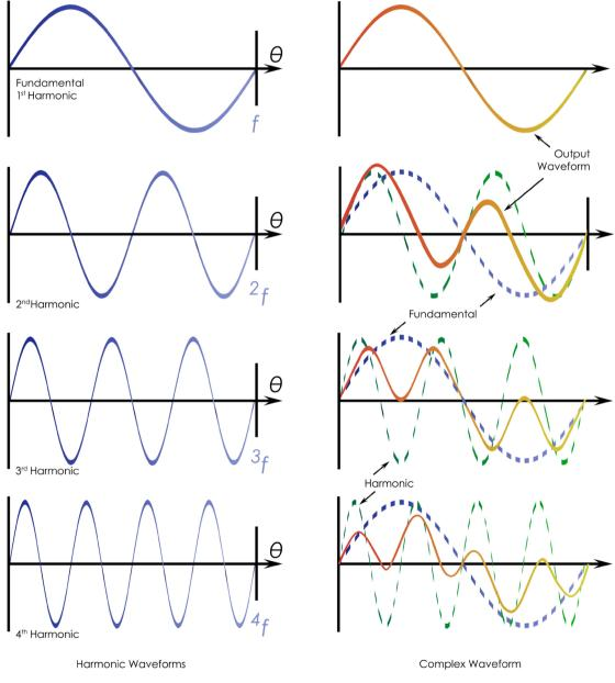
Figure 2. Typical harmonic waveforms.
