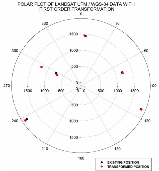
Figure 8. Polar plot of Landsat UTM/WGS-84 data with first order transformation.
