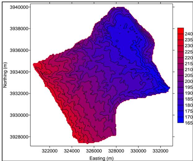
**Figure 3.** 2D elevation model of the area of salt ponds, typical area for salt product marked by blue color, (extracted by Global Mapper v10 from N35-E43-hgt file, and exported as grid file to SURFER-8).
