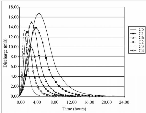
Figure 3. NRCS Unit Hydrographs of Makkah' Catchments.
