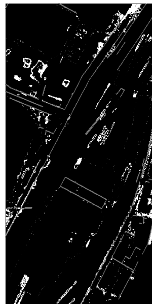
Figure 9. Comparison between the extracted features and 1:1000 digital maps of Milan. In red the wall features manually extracted. We can observe a good result for 50% of elements, while some walls are not recognized and we have many false-positive due to the presence of many objects which have wall's similar characteristics.
