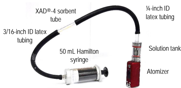
Figure 1. Apparatus set-up for aerosol sampling consists of 50 mL Hamilton air-tight syringe, latex tubings, XAD®-4 sorbent tube and e-cigarette devices.
