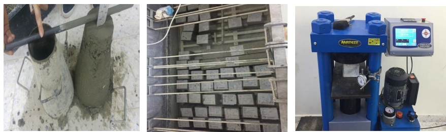
Figure 2. Slump test, curing and compressive stress tests of concrete.
