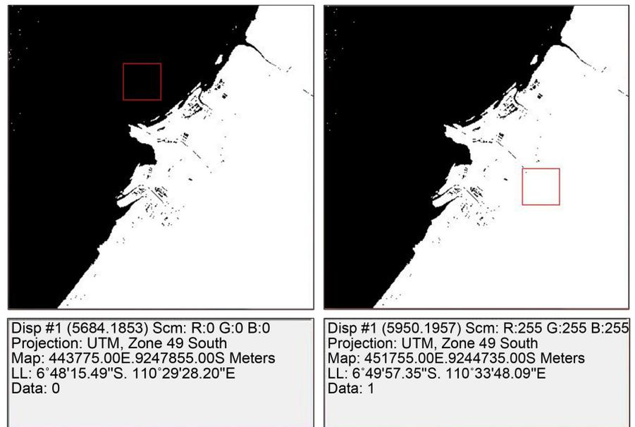
**Figure 2.** Results of Landsat ETM imagery processing using the histogram threshold method in which 0 represents the sea (left) and 1 describes the land (right).
