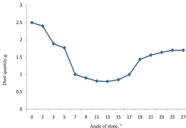
**Figure 2.** Dependence of dust quantity on the angle of slope of conveyer (concentration of RCOOCu solution—0.13%).
