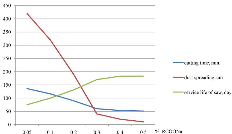
**Figure 1.** Dependence of parameters of stone-cutting process on the concentration of RCOONa in solution.
