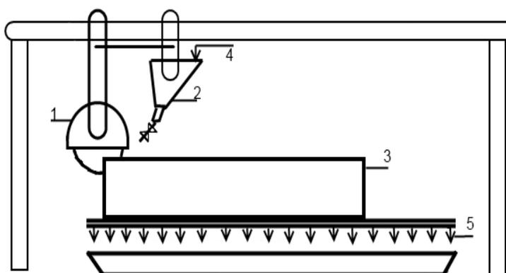
**Figure 3.** A schematic diagram of installation for dust minimization in stone quarry. 1. Stone-cutting instrument; 2. Funnel for naphthenate solution supply; 3. Stone; 4. Naphthenate solution; 5. Vessel for gathering dust-naphthenate mixture.
