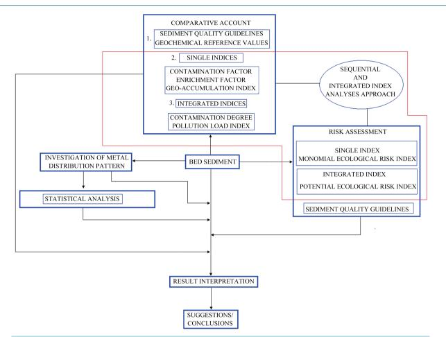
Figure 2. A schematic representation of methodology employed to characterize Subarnarekha bed sediments.
