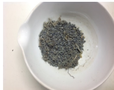
Figure 5. Close appearance of removed lead sinker.
