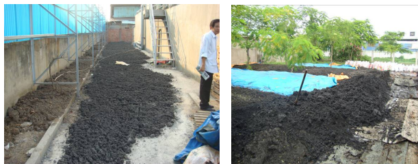
Figure 3. Sludges generated from the wastewater treatment plant of Din Ki tanneries and Le Minh Xuan Industrial Zone (4000 m 3 /day).
