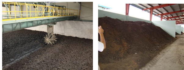
Figure 2. Sludges generated from the Binh Hung wastewater treatment (141,000 m 3 /day) before/after treated by composting plant.
