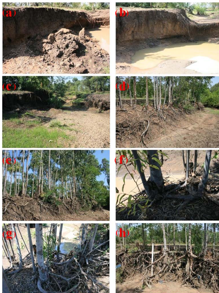
Figure 1. Field survey of Eucalyptus root system and its performance in blocking gully erosion development at Kokal village in Kisumu, western Kenya. Slumping of gully walls occur in the absence of Eucalyptus roots (a)-(c). Eucalyptus root system hold large soil mass preventing slumping of gully walls (c)-(e). Eucalyptus roots fused forming intimate mass of root system (f), (g). Neighboring Eucalyptus supported adjacent tree whose roots were freed of soil by water erosion (h).
