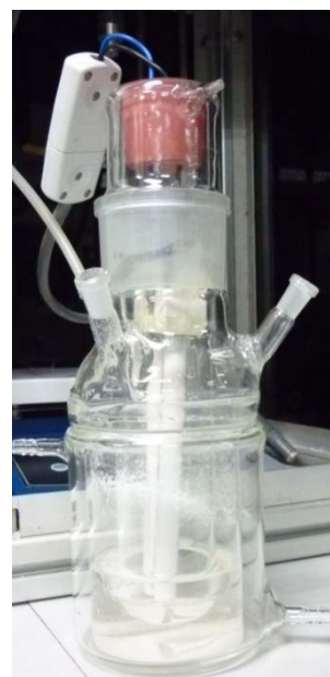
Figure 2. The view of the photo-reactor used.
