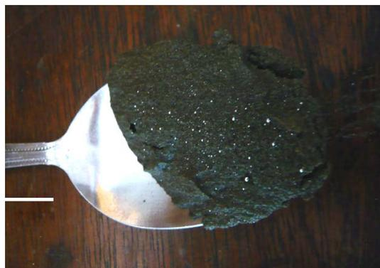
Figure 1. Mercury flour in tailings. Scale 1 cm.
