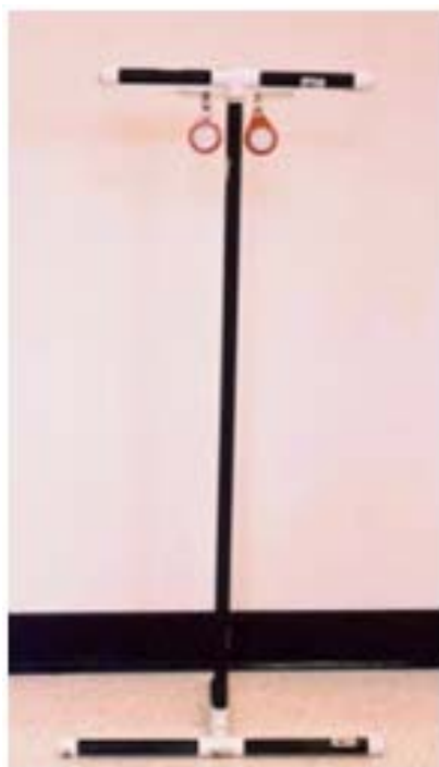
Figure 3. Indoor stand for monitoring of VOCs.
