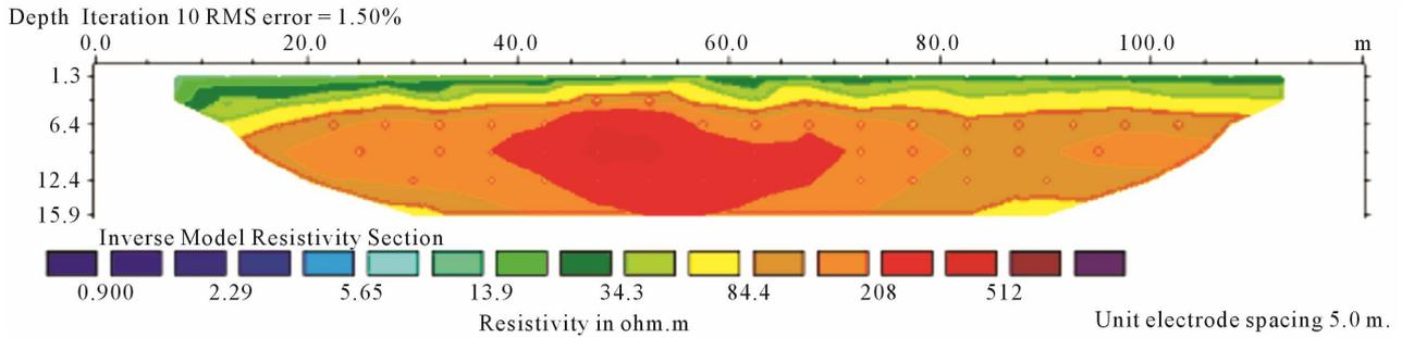
**Figure 4. 2-D electrical image section of line PS1 (A).**
