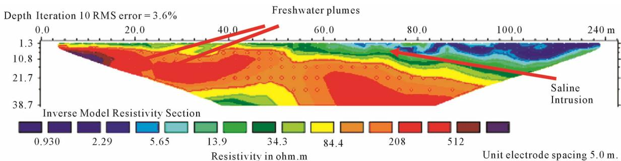
**Figure 7. 2-D electrical image of line PS4 (D).**
