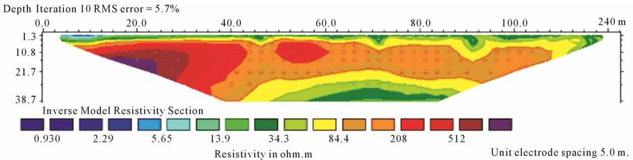
**Figure 6. 2-D electrical image of line PS3 (C).**
