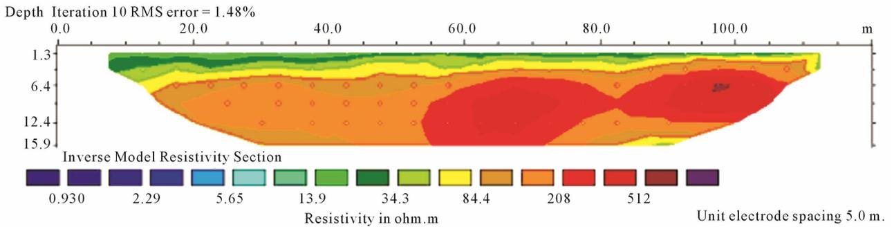
**Figure 5. 2-D electrical image of line PS2 (B).**
