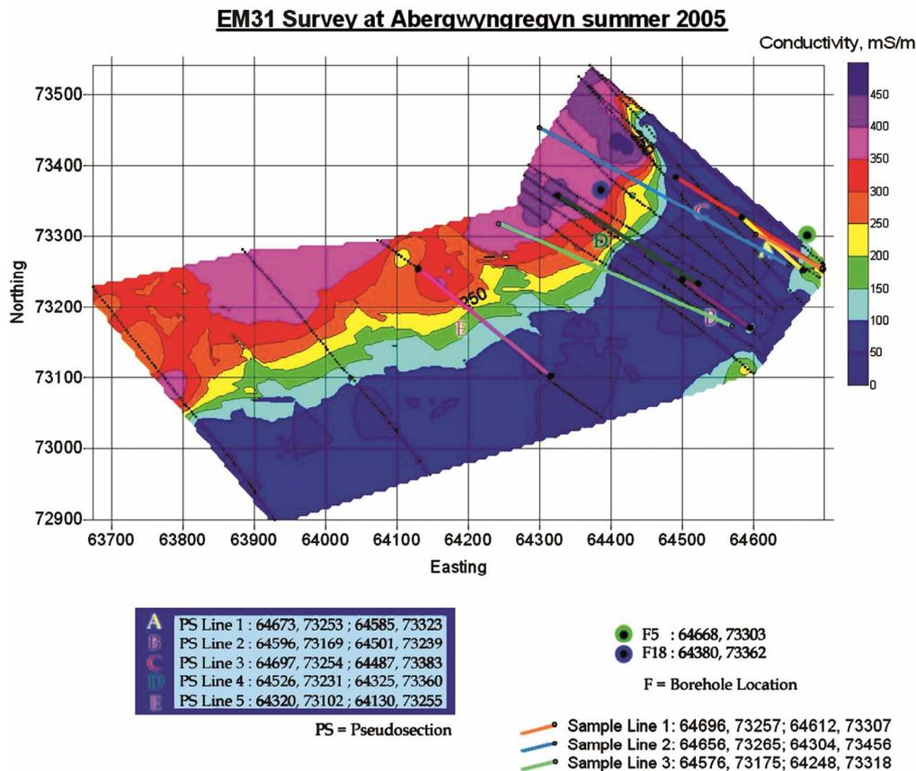
**Figure 3.** EM31 conductivity contour plot with pseudo-section lines; sample lines and borehole points superimposed.
