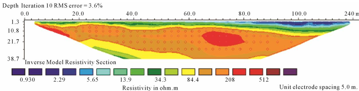
Figure 8. 2-D electrical image of line PS5 (E).
