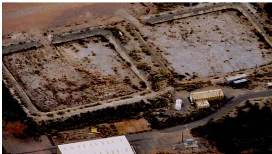
Figure 6. Evaporation beds for disposal of pesticide wastewater [43].
