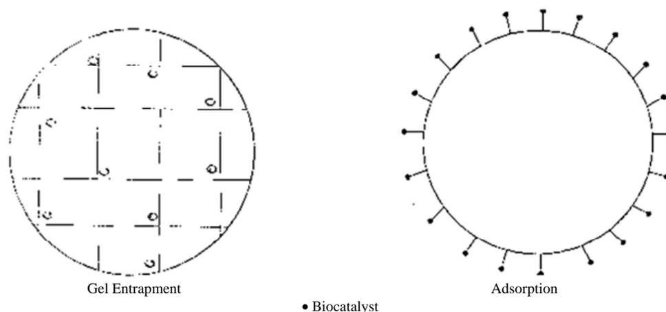
**Figure 1. Approaches of immobilized biocatalysts.**
