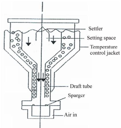
Figure 10. Airlift loop reactor with draft tube as downcomer.
