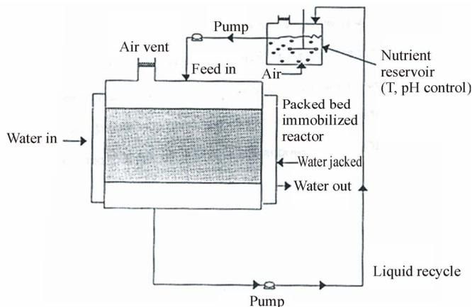
Figure 12. Packed bed reactor.
