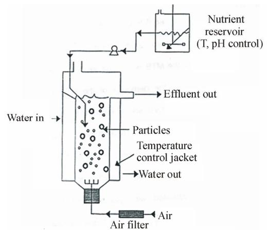
Figure 11. Fluidized bed reactor.
