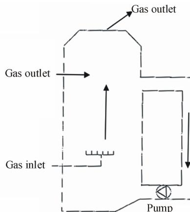
Figure 6. Pumped tower loop reactor (PTLR).
