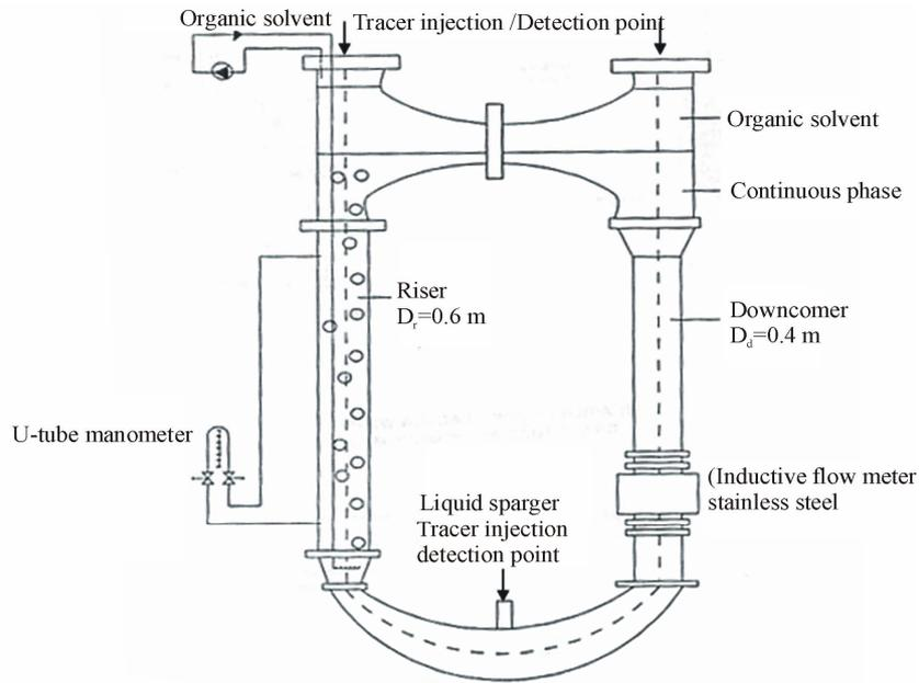
Figure 7. Liquid impelled loop reactor (LILR).
