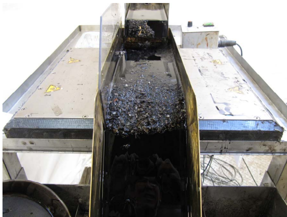
Figure 2. Equipment for MDS separation of aluminium (floating) from heavy non-ferrous metals (sunk and collected at bottom of the gutter).
