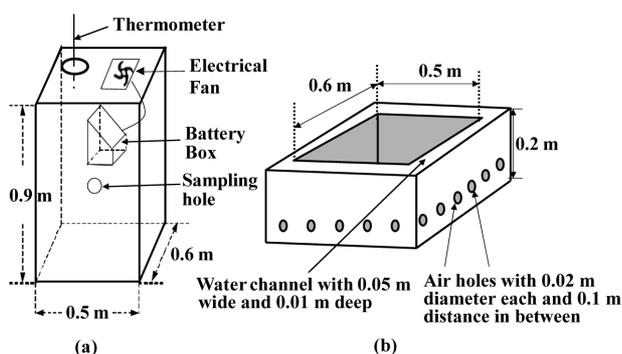
**Figure 1. Experimental set up for collection of CH<sub>4</sub> gas. (a) the gas chamber and (b) the aluminum alloy base.**
