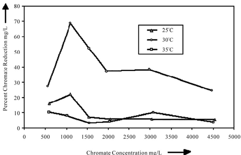
Figure 2. Effect of initial Cr (VI) concentration on Cr (VI) removal by *Bacillus circulans* MN1 at 25°C, 30°C and 35°C respectively.
