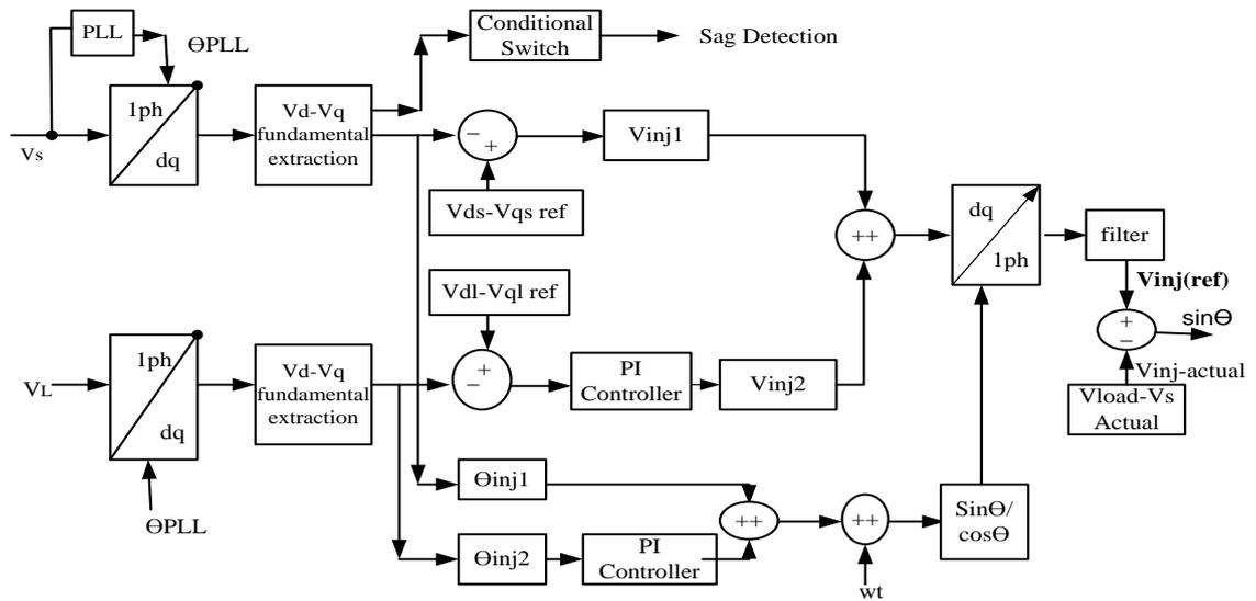
Figure 4. MATLAB based model of proposed control method.
