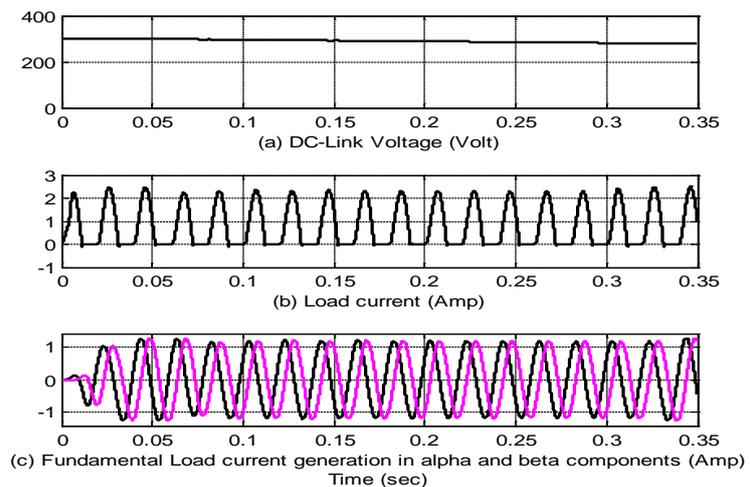
**Figure 9.** DC-link voltage and load current in case of nonlinear load.
