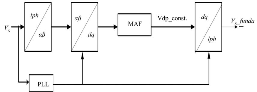
**Figure 2.** Fundamental positive sequence component extraction.
