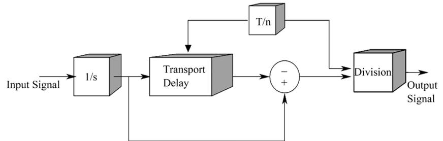
**Figure 3.** Block diagram of the moving average filter (MAF).
