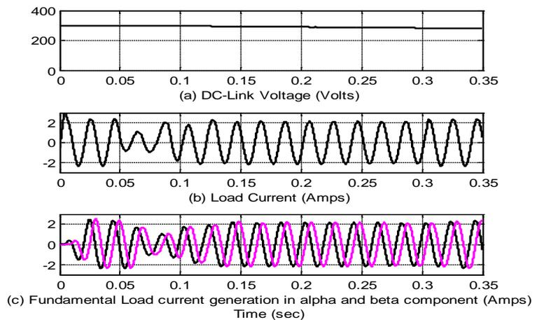
Figure 7. DC-link voltage and load current in case of linear load.
