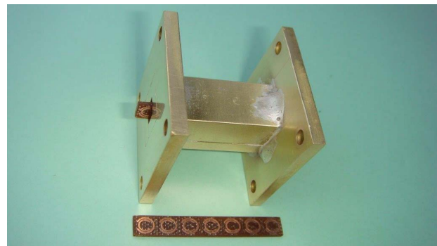
Figure 4. Waveguide loaded with split-ring resonator.
