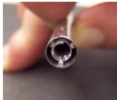
Figure 5. Photo of the assembled helix circuit with three support rods inserted in a stainless steel shell using a triangulation method.
