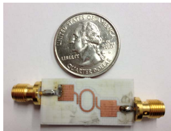
Figure 8. Fabricated elliptical patch resonator bandpass filter.
