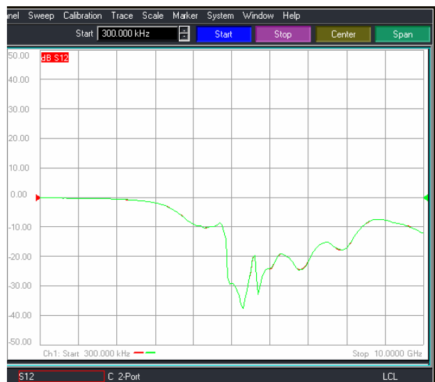
Figure 12. Measured S_{21} response for conventional Low pass filter.
