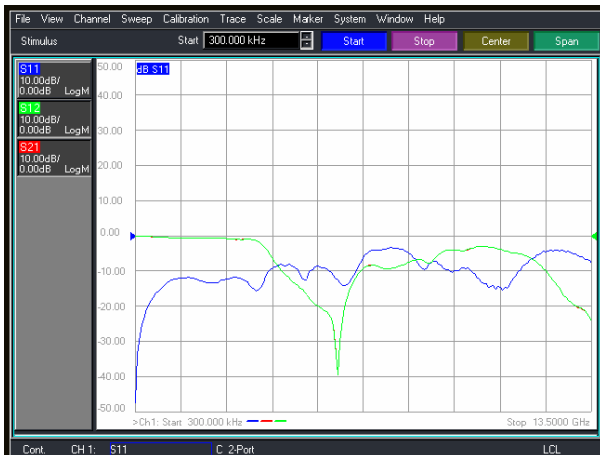
Figure 13. Measured S_{21} & S_{11} response for low-pass filter with 5 hex-omega particles etched into the ground plane.
