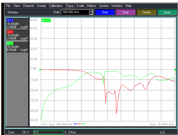
Figure 14. Measured S_{21} & S_{11} response for the proposed low-pass filter with 4 hex-omega particles etched into the ground plane.
