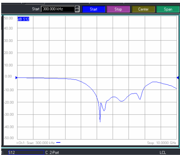
Figure 15. Measured S_{21} response for the proposed low-pass filter with 3 hex-omega particles etched into the ground.
