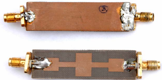
Figure 10. Picture of fabricated conventional maximally flat. (a): bottom & (b): top of low-pass filter.
