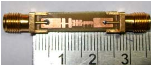
Figure 2. Snap shot of fabricated bandpass filter.
