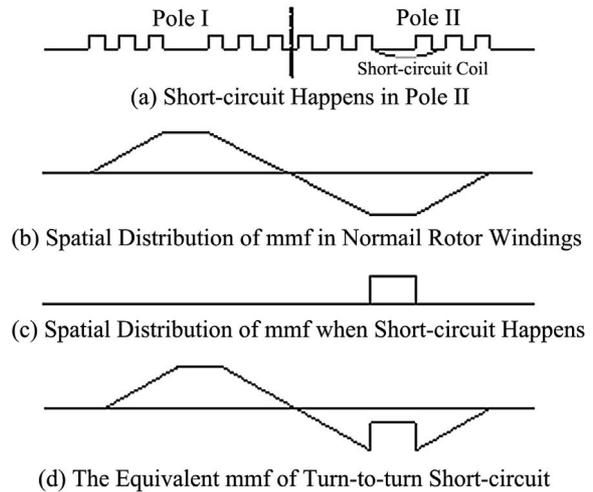
Figure 1. Spatial distribution of mmf in rotor windings
