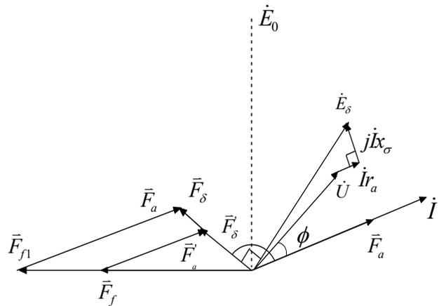
Figure 2. Magnetic-electronic potential vector of generators considering saturation
