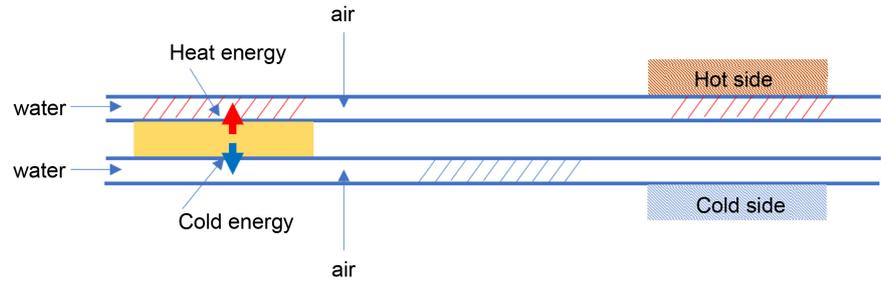
**Figure 2.** Design of electrocaloric cooling system.
