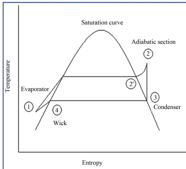
**Figure 4.** Thermodynamic operation of heat pipe.
