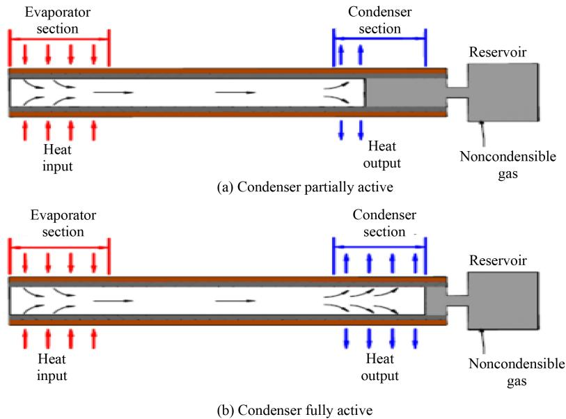
**Figure 6.** Variable conductance heat pipe.
