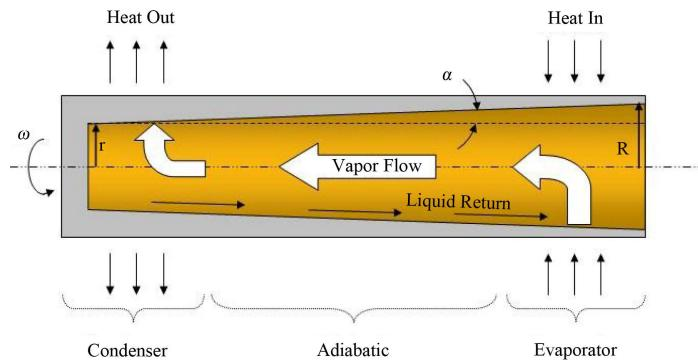
**Figure 8.** Flow mechanism in a rotating heat pipe.
