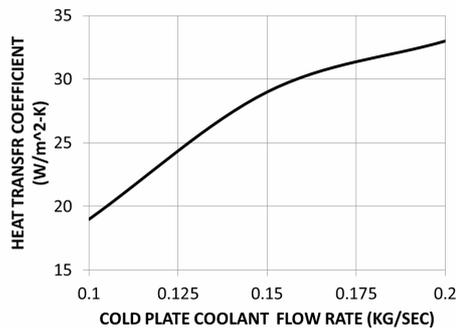
Figure 14. Heat Transfer coefficient versus cold plate flow rate.
