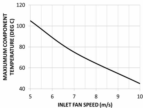
**Figure 19.** Maximum component/chip temperature versus cooling fan inlet air speed.
