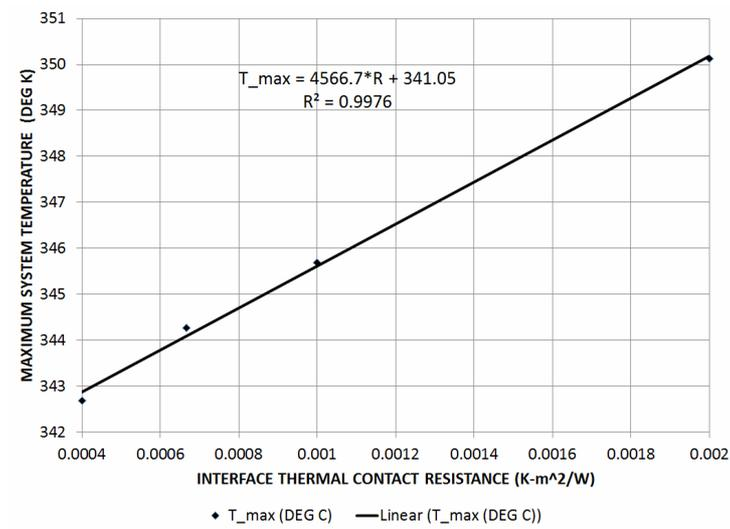
Figure 16. Thermal fault simulation showing effect of contact resistance.
