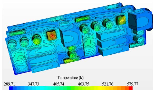
Figure 18. Thermal fault simulation of defective chip.
