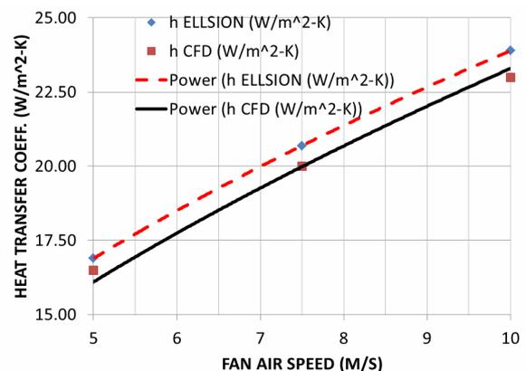
Figure 12. Heat transfer coefficient versus fan air speed.
