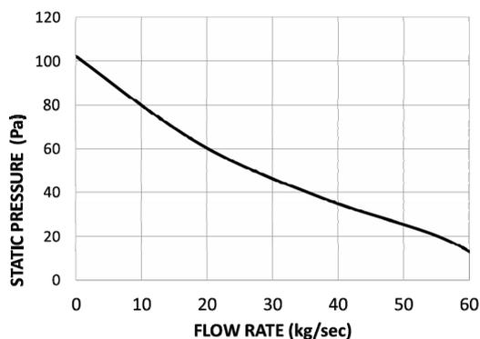
Figure 3. Fan curve specifications for thermal control hardware simulations.
