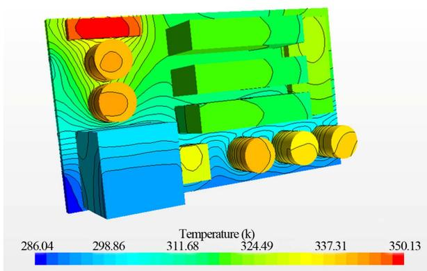
Figure 17. Effect of poor thermal contact resistance.
