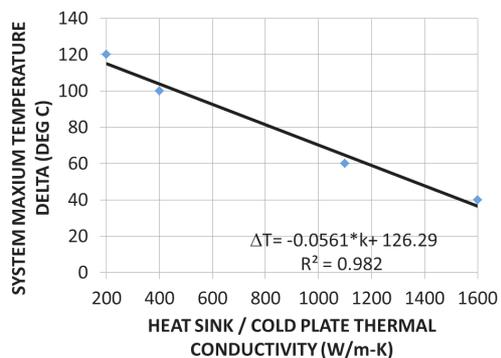
Figure 10. Thermal conductivity effect on heat spreading in CFD simulations.
