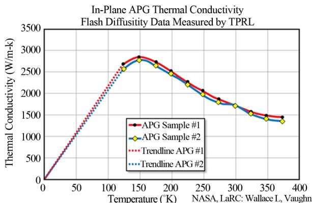
Figure 2. Thermal conductivity for APG material [1].
