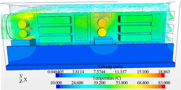
Figure 8. Velocity vectors colored by air speed and electronics components colored by temperature.
