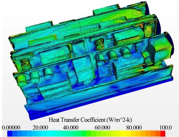
Figure 11. Convective heat transfer coefficient contours.
