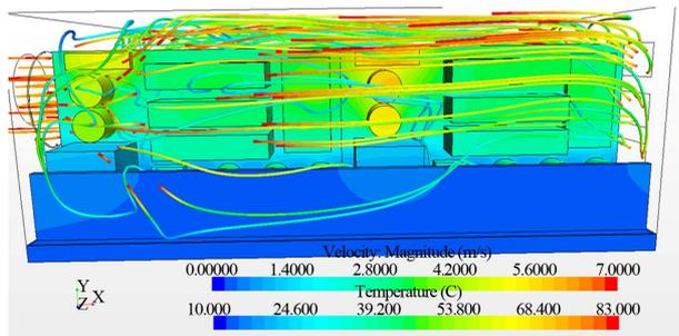
Figure 9. Streamlines colored by air stream speed and electronics components colored by temperature.
