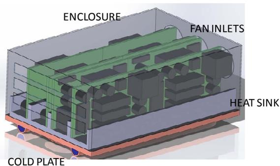
Figure 4. Electronics System Components.
