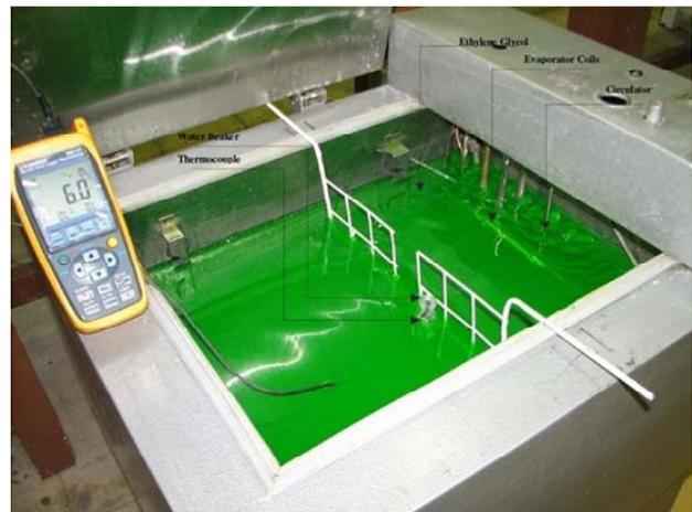
**Figure 1.** Cold bath with ethylene glycol as the freezing media.
