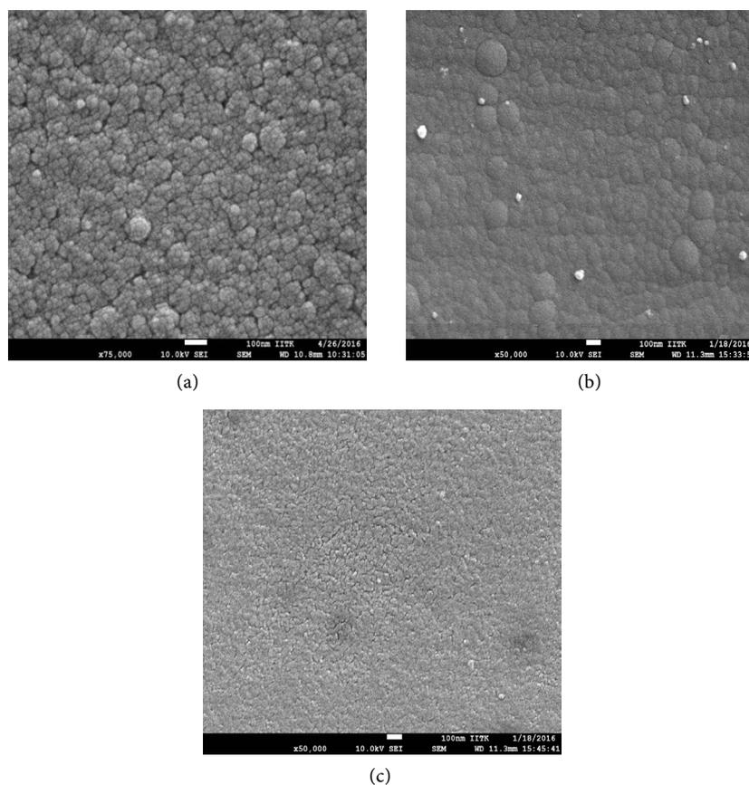
**Figure 4.** SEM images of (a) SiO<sub>x</sub>; (b) SiN<sub>x</sub> and (c) SiN<sub>x</sub> over SiO<sub>x</sub>.
