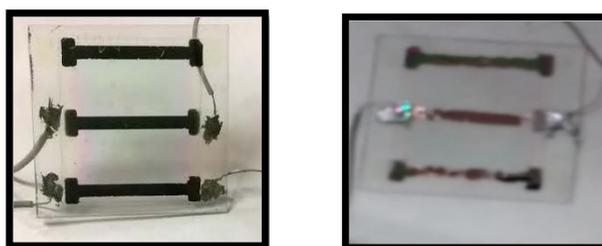
**Figure 1.** Encapsulation experiments of calcium test lines (black).
