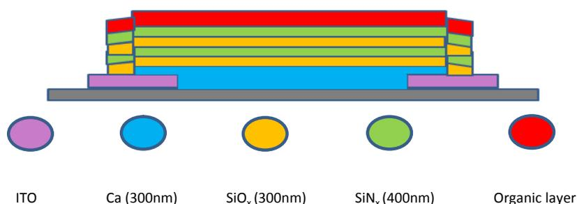
**Figure 3.** Schematic of the two inorganic dyads/acrylic encapsulation of Ca test structure.
