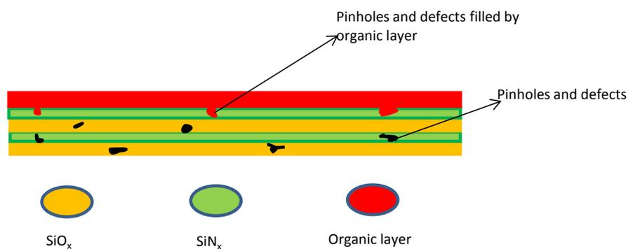
**Figure 5.** Filling of defects of inorganic layer using organic layer.
