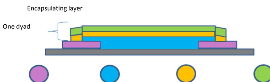
**Figure 2.** Schematic of the inorganic dyad encapsulation of Ca test structure.
