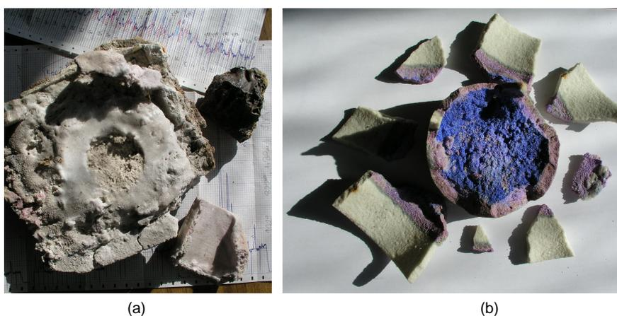
**Figure 1.** The appearance of the linings of cooking stoves (a) and security of the crucible (b) after melting slag I.
