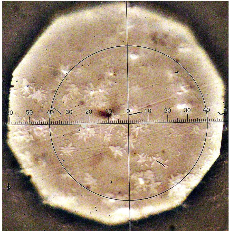
**Figure 13.** Optical photo of crystals of magnesiochromite (white centers) and diopside of outlet in glass I a. Thermal history: 740°C 4 h - for the nucleation of magnesiochromite and 750°C for 4 h + 880°C 20 min - for the nucleation and development of diopside. Graduation is 1  $\mu$ .
