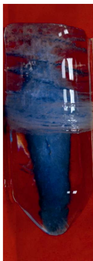
Figure 3. Bromthymol blue solution after crystallization in tube. Pure ice on the border of the tube and the blue solution at its center is seen on the red background. In the course of crystallization the component was displaced from the solid into liquid phase.
