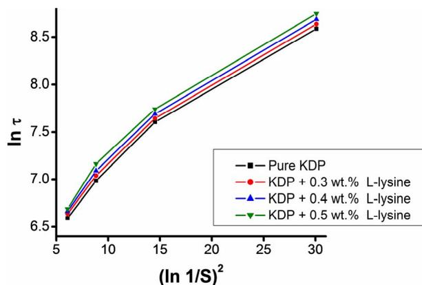
**Figure 4.** Plots of  $\ln \tau$  versus  $1/(\ln S)^2$  for pure and, L-lysine doped KDP crystals.
