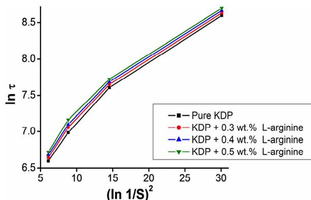
**Figure 3.** Plots of  $\ln \tau$  versus  $1/(\ln S)^2$  for pure and L-arginine, doped KDP crystals.
